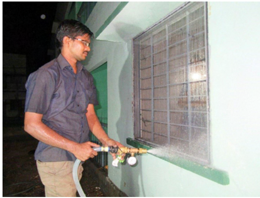
Fig. 4.21: Water pressure test for window joint
