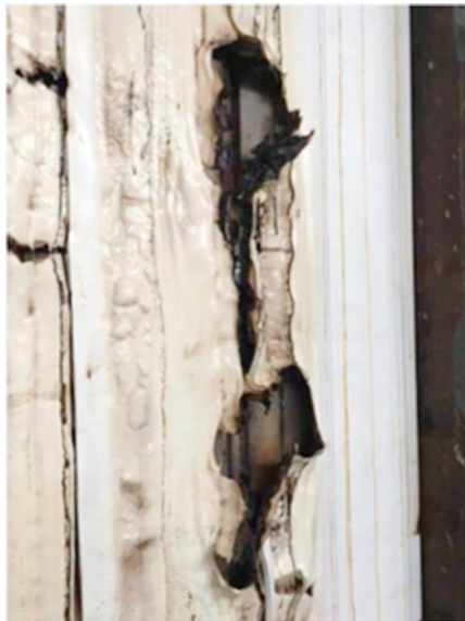
Fig. 4.11: Failure of PVC panels during fire testing [6]
